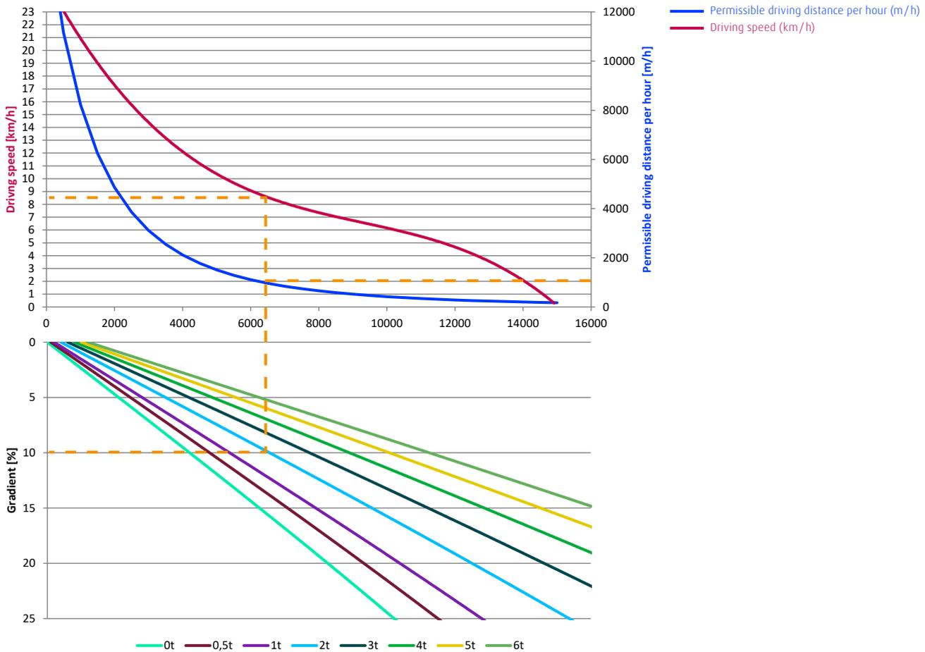
The example shown illustrates a load transporter transporting 2 t operating on a ramp of 10 %, maximum travelling speed reachable 8.5 km/h for a maximum travel distance per hour of 1.6 km (1600 m\*)
