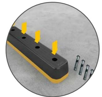
The StepBumper is easy to install with a maximum of 4 x M16 – OD24mm Bolt Type Head fixings (1200mm version) per Step Guard. This means that the product can be installed or replaced quickly with a minimum amount of disruption on site.
